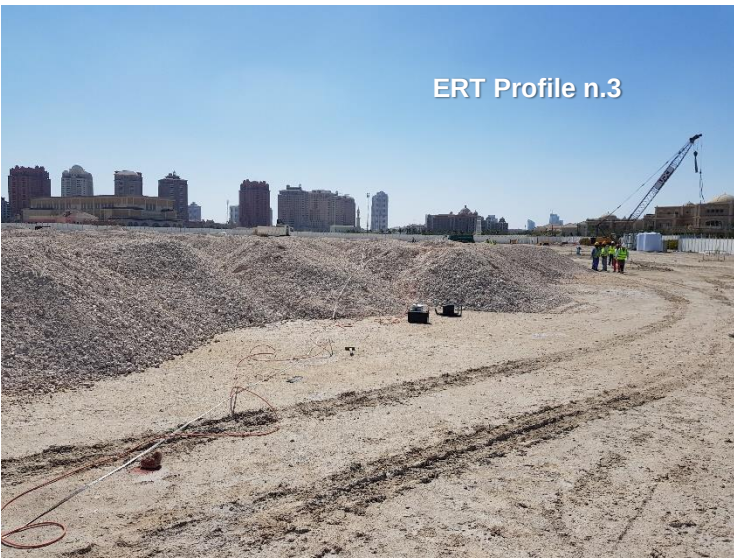
Resistivity Device, center of the ERT profile
